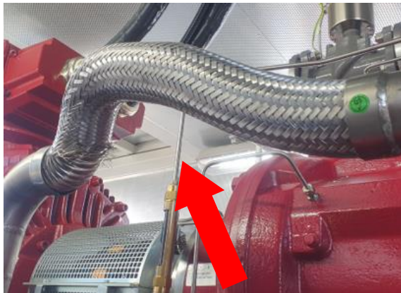
Figure 1 (left side) Burst hydraulic oil hose after the event. The installed hose was too long. (See Figure 3).
